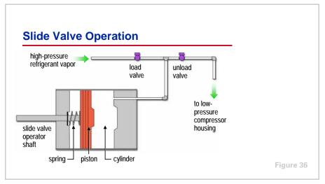
The slide valve is operated by a piston and cylinder assembly. Extension and retraction of the operator shaft positions the slide valve along the compressor rotors.
